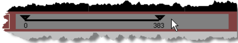
Figure 1.23 Use the W/L Slider to adjust the Window Width (left slider) and the Window Level (right slider).
